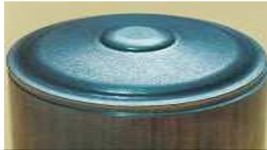
Shock Absorber 25000J Pressure tight weld of an endcap to a shock absorber tube Material: FeC to FeC
