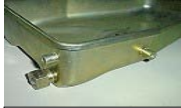
Oil Sump 25000J Pressure tight welds of connection studs to an oil sump body Material: FeC to FeC
