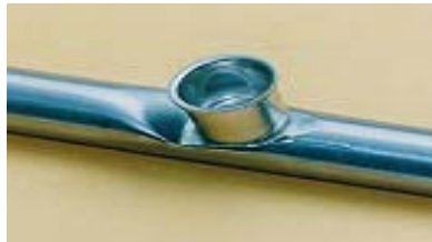
Fuel Connection Stud 500J Fixing of the connection stud to the tube prior to soldering Material: CrNi to CrNi stainless
