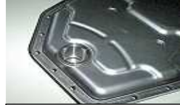
Oil Sump Bottom 25000J Pressure tight weld of an outlet stud to an oil sump body Material: FeC to FeC
