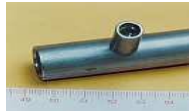
Hydraulic Cylinder Connector 6000J Pressure tight weld of a stud to a hydraulic cylinder tube Material: FeC to FeC
