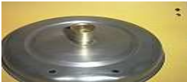
Water Inlet 15000J Pressure tight weld of a brass stud to a steel body plate
