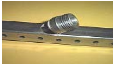
Gas Distributor 15000J Gas tight weld of a connection stud to a tube Material: FeC to FeC
