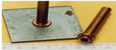
Compressor Connector 6000J Weld of a copper tube to a steel housing (watertight)
