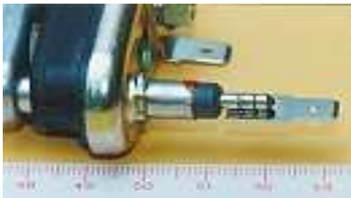
Heater Connector 500J Weld of a flat connector to a round material without influence of the heat sensitive isolator material Material: FeC to CrNi
